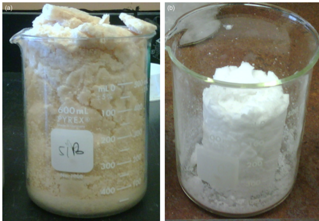
Fig. 1. Foam products from the esterification sol-gel synthesis: (a) as-synthesized organic foam, and (b) oxide composite foam produced by calcining the sample from (a) in air at 400°C for 24 h.
